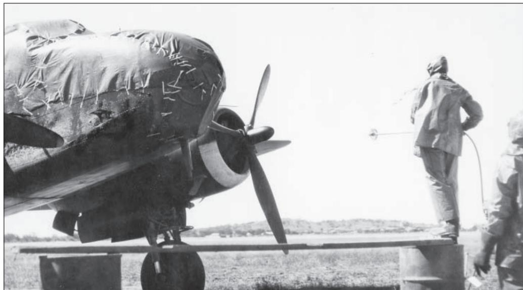
A bomber is sprayed with mustard gas in an experiment to determine the effect of the gas in flight. Top, decontamination is carried out fore crew and scientists after the flight.
